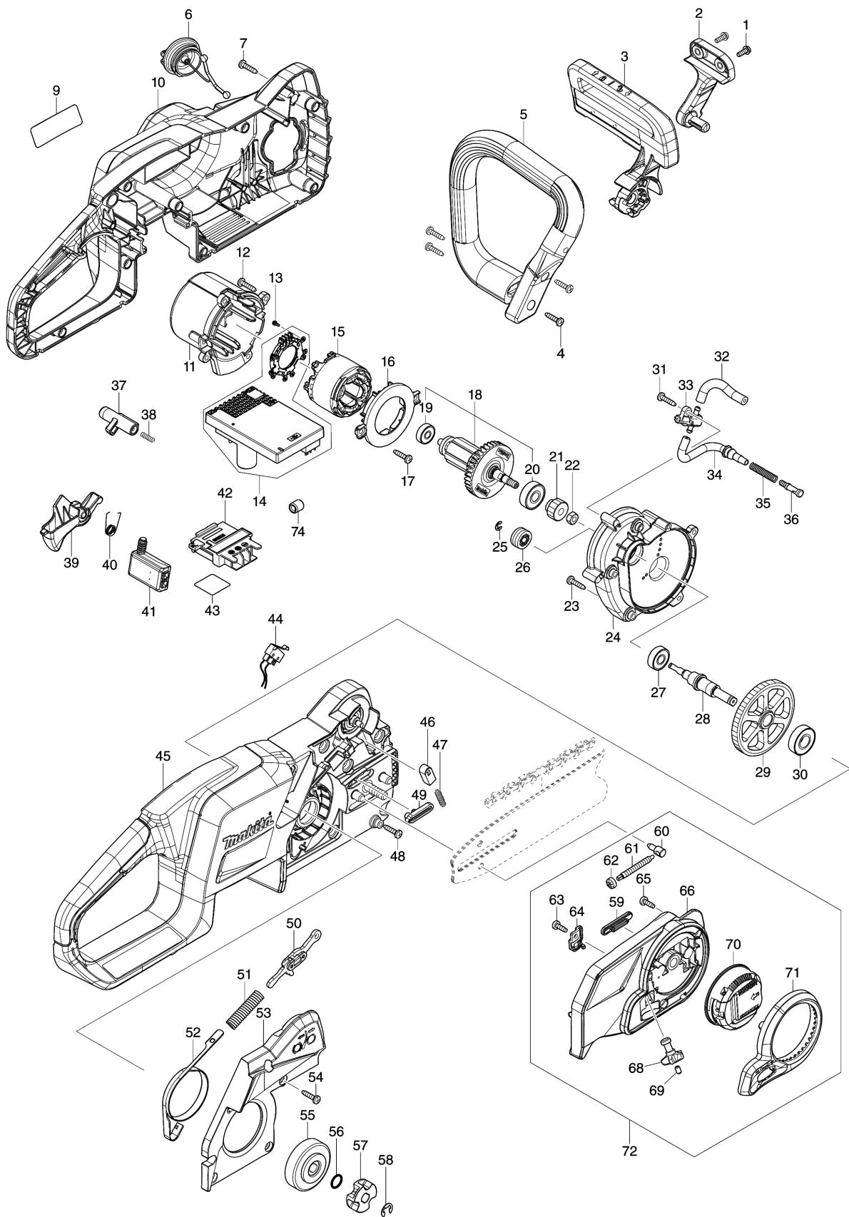
**Model No.DUC407 400MM CORDLESS CHAIN SAW**
