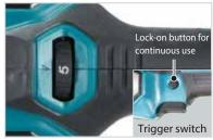
Setting up RPM at full up position of trigger is easy by a variable speed dial. Variable speed control by trigger enables to adjust RPM during operation.
